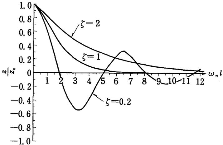
Fig. 14.2 Motion of liquid column with frictional resistance
