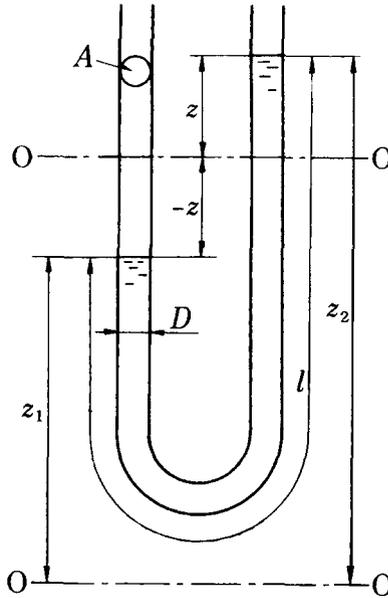
Fig. 14.1 Vibration of liquid column in a U-tube
